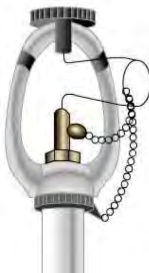
Figure 4-10 – Sprinkler pre-prime plugs.
